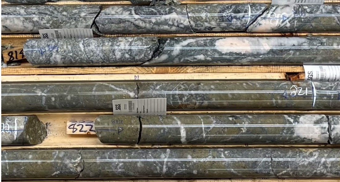
Image 3: Representation of mineralized and altered porphyry core from DQ23-02 (25.0 m of 1.69 g/t Au); bottom of hole ended in mineralization and this zone is subsequently being extended by additional drilling.
