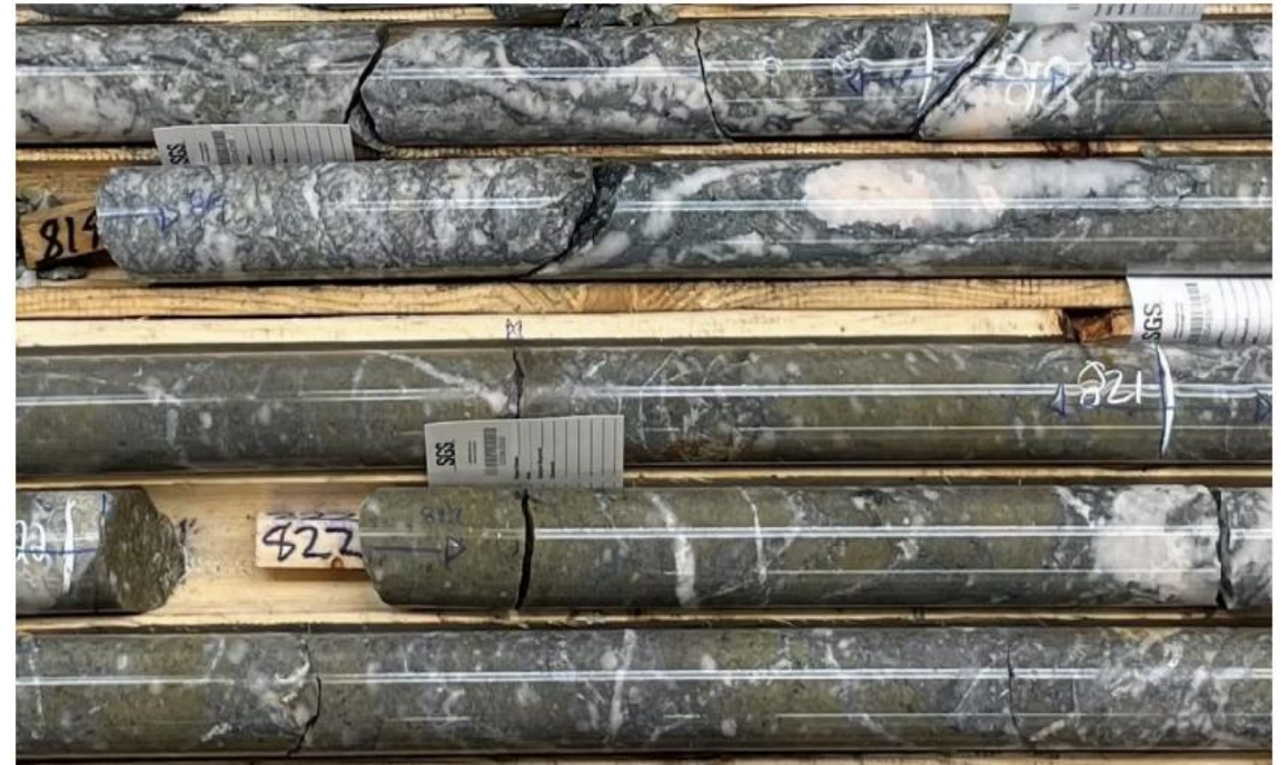
Representation of mineralized and altered porphyry core from DQ23-02 (25.0 m of 1.69 g/t Au) ; bottom of hole ended in mineralization and this zone is subsequently being extended by additional drilling. – core depth of 814 m
